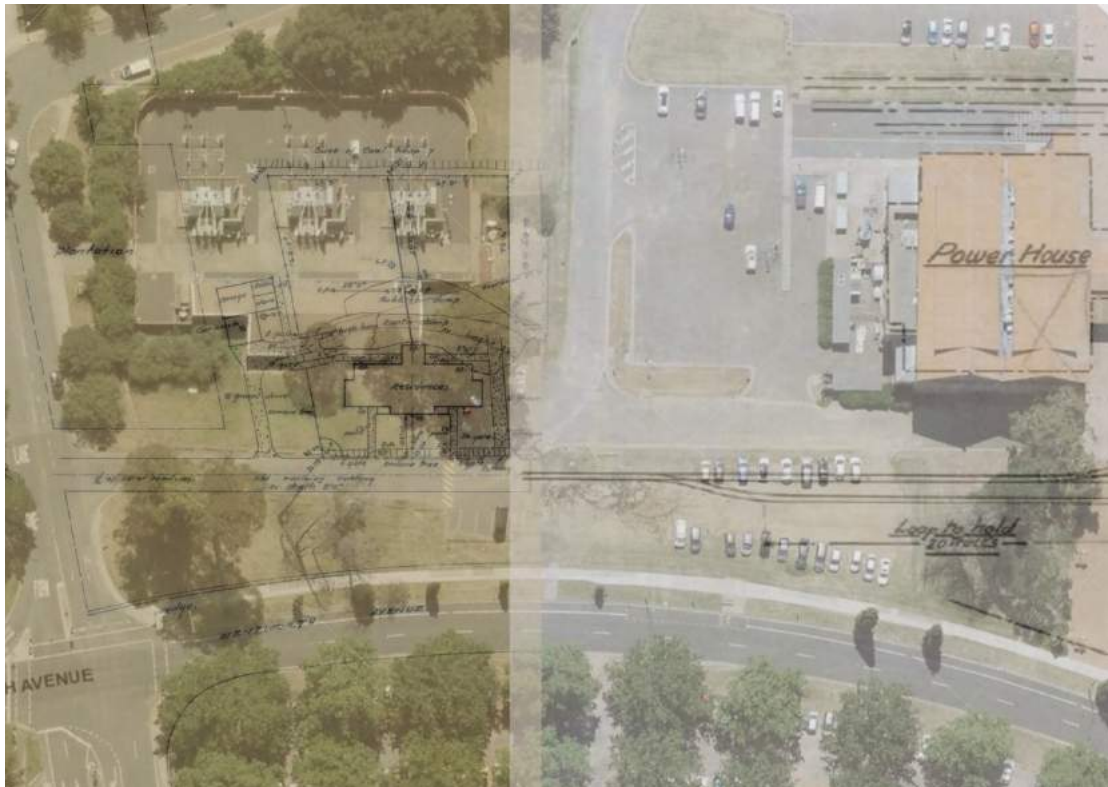
Overlay showing the approximate location of the brickworks railway and circa 1941 roadway relative to the current vehicle entry from Eastlake Parade. The drawing on the left side indicates that the road for residences was constructed on the brickworks railway cutting. The current entry to the car park is in a similar location. (Source: National Archives of Australia A2617, Section 59/13802 and A2445, M2270C overlaid on ACTmapi aerial, showing February 2022)
