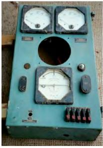
Control and Synchronising Switchboard Salvaged from 1953 Kingston Diesel Auxiliary Station
