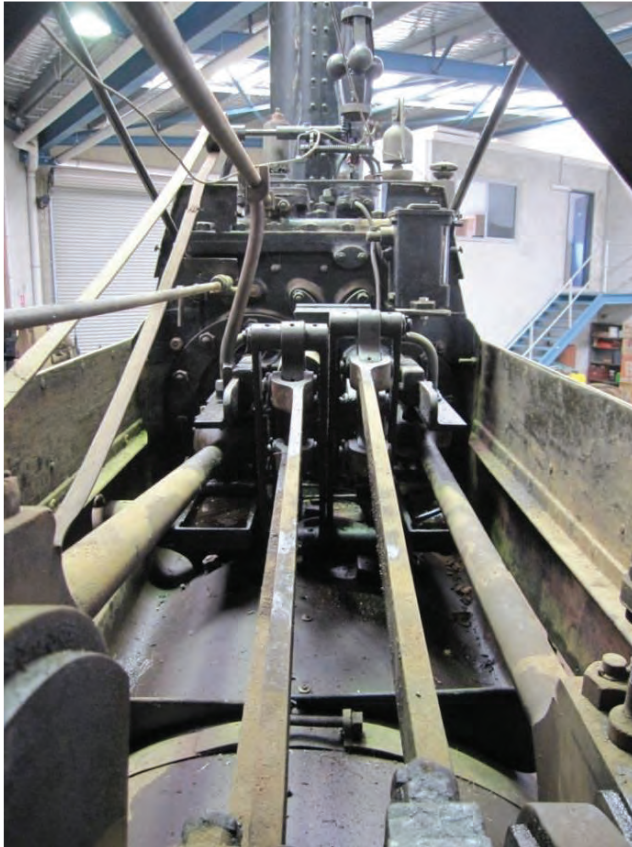
Figure 29 Engine on top of the boiler looking forward towards the cylinder with the Stephenson's reversing links in the middle Source: Rohan Lamb, December 2013
