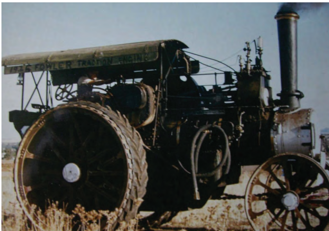
Figure 20 Fowler no.16161, shortly after conservation works by Bob McLeod, c.1963: note the short cut out section in the front edge of the original canopy Source: Bob McLeod collection
