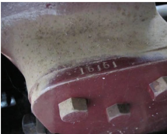
Figure 27 Left and right: Engine serial number 16161 stamped into the edge of the spectacle plate Source: Rohan Lamb, December 2013
