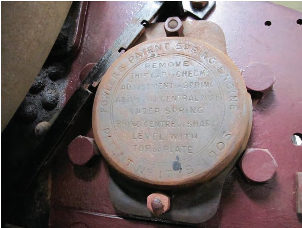
Figure 32 Rear axle spring adjustment cover: note the reference to patent no.1775-1903 Source: Rohan Lamb, December 2013
