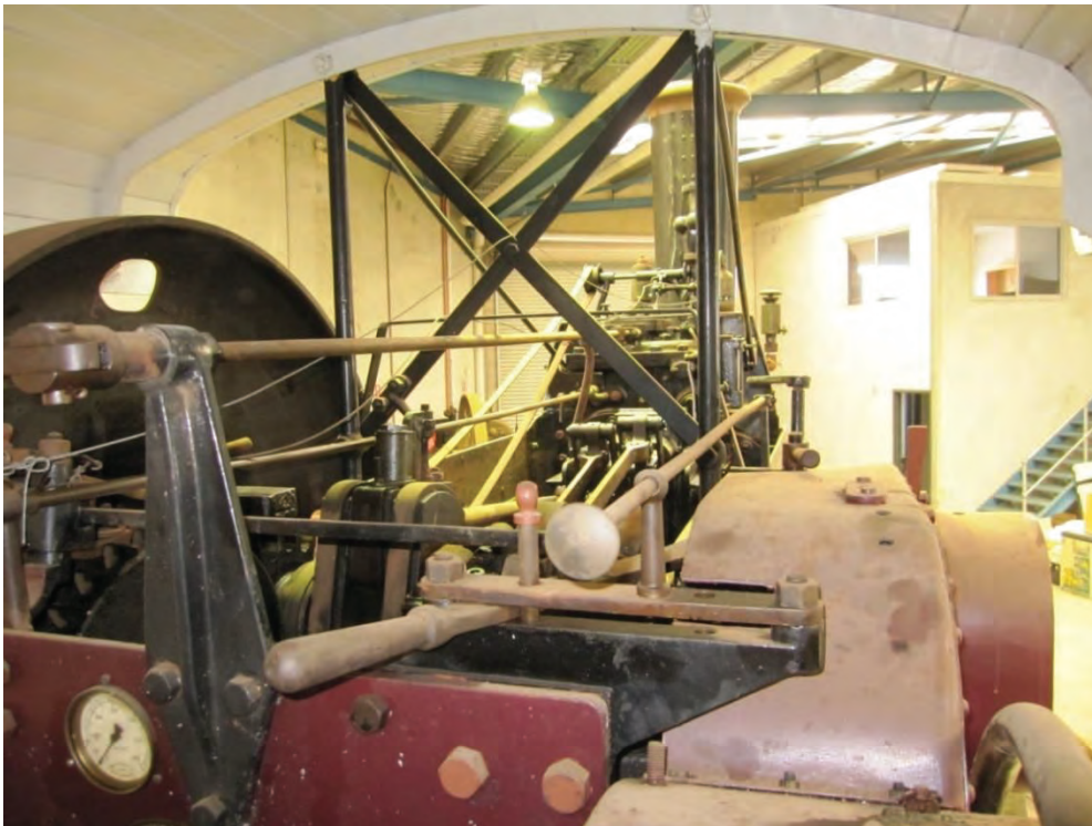
Figure 39 View from the footplate showing the driving levers and engine Source: Rohan Lamb, December 2013
