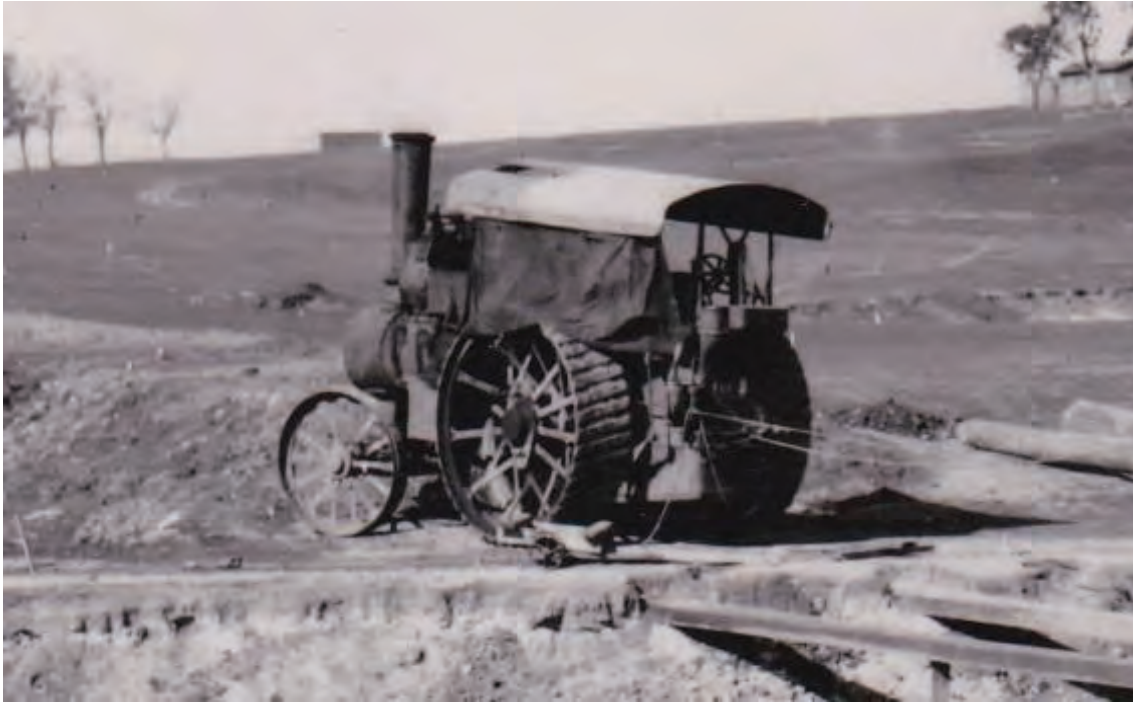
Figure 18 Close up view of Fowler road locomotive no.16162 showing the slot in the canopy above the flywheel
