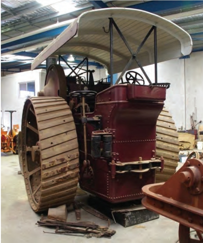
Figure 38 Rear view showing rear tender, hand brake, and canopy Source: Rohan Lamb, December 2013
