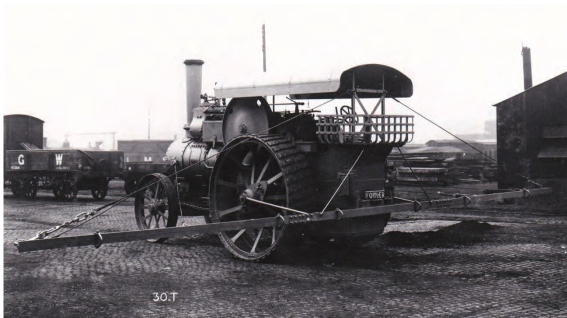
Figure 43 Fowler no.16163 in Fowler's yard, Leeds with the 40' (12.2m) draft beam in place Source: Museum of English Rural Life
