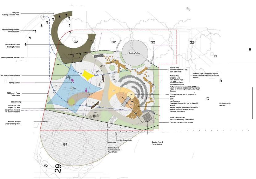
Legend 0 Existing Trees Grey Concrete Paths Oxide Coloured Concrete Bark Softfall Mass Planting Bed Mulch Only Rubber Softfall Permeable Paving 1200mm H Fence / Gates Timber Log Seats Debarked Timber Logs Timber Log Steppers Mixed Heights: Flush With Ground + Up To 0000 300mm H 150mm Min To 300mm Ø Stone Stepping Pavers Stone / Rock Bank Seat
