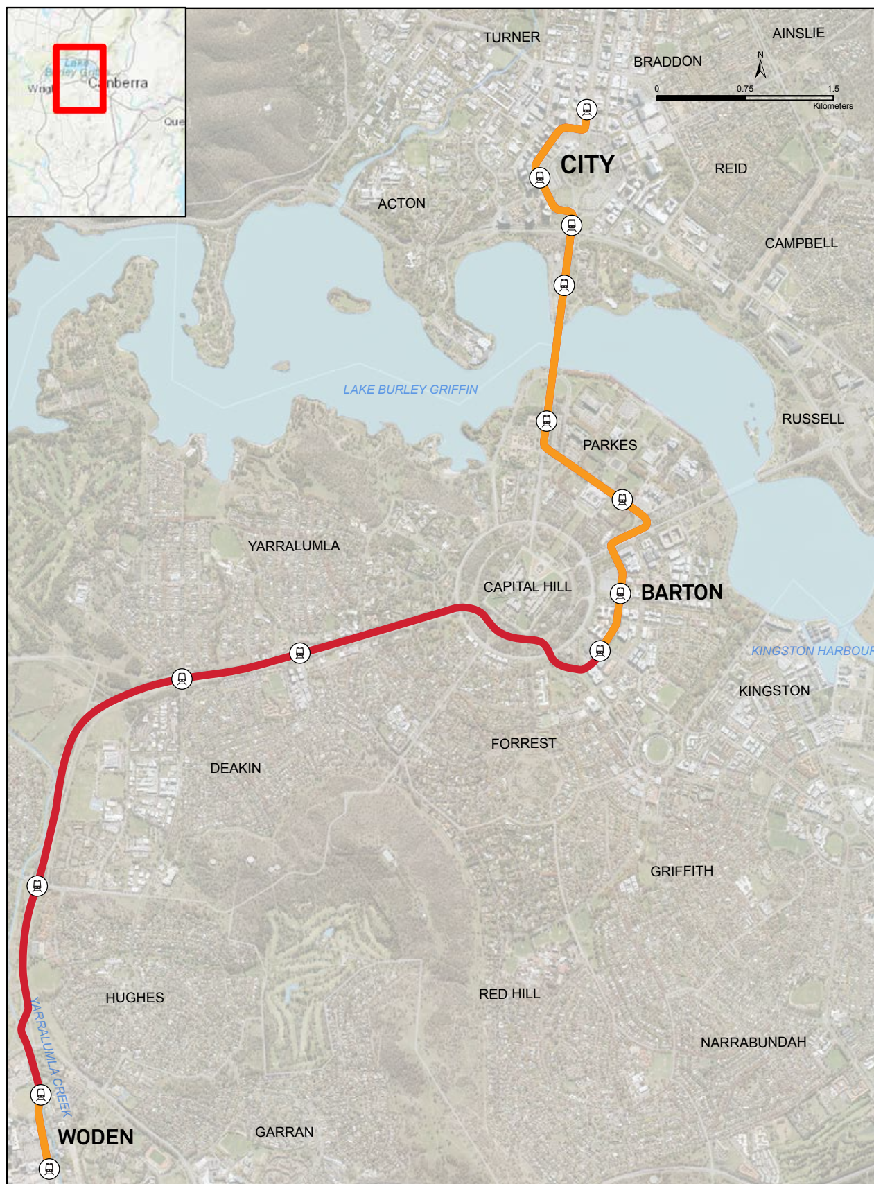
Figure 18: Overhead line power and wire-free running locations
