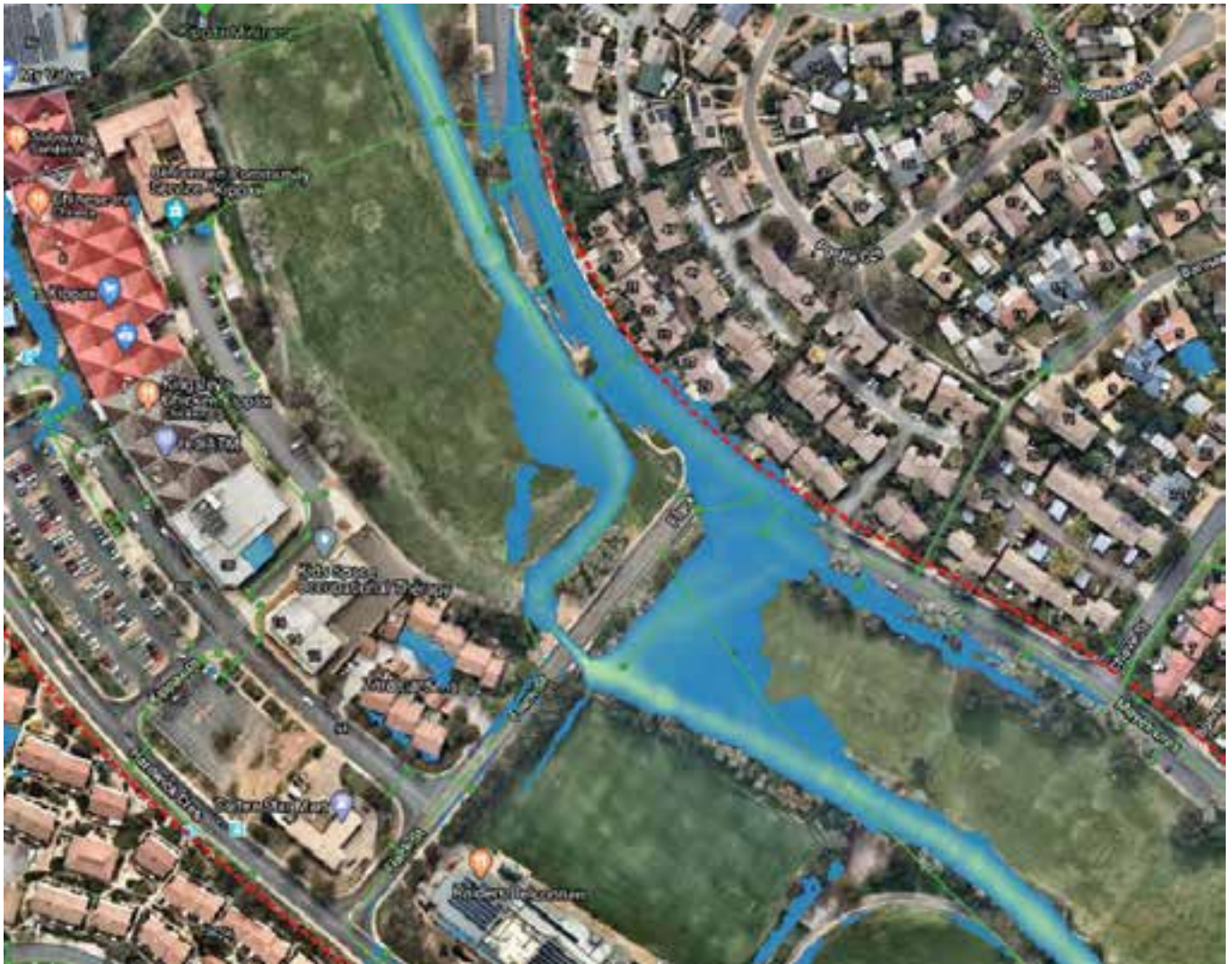
Figure 8-6: Peak flood levels at Flack Street during a 1% AEP 25 minute storm event
