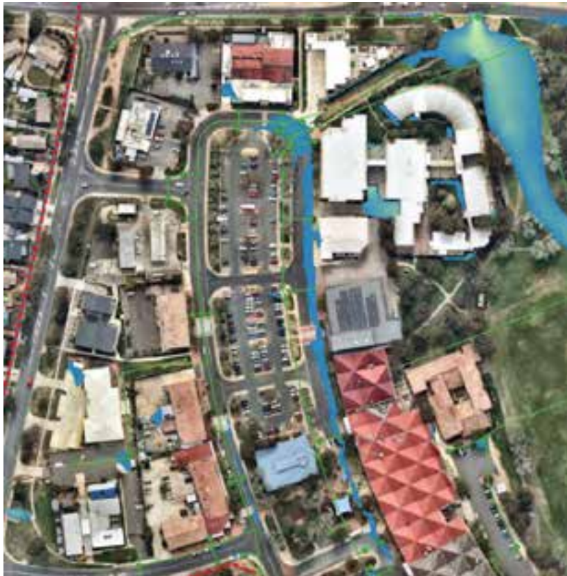
Figure 8-2 Peak flood extents along Hardwick Crescent during a 20% AEP 25 minute storm event
