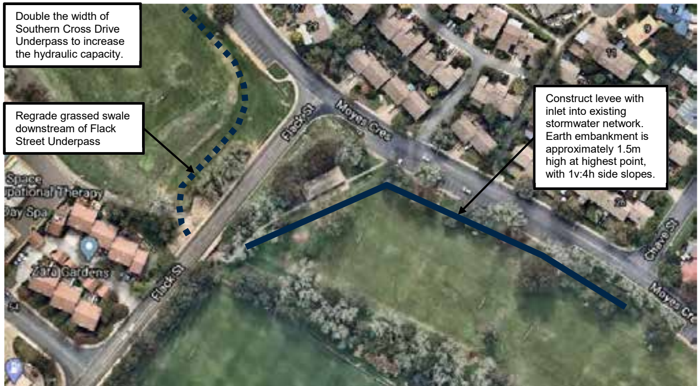
Figure 10-1 Mitigation Option – Channel regrading, and levee at Flack Street and Moyes Crescent Intersection
