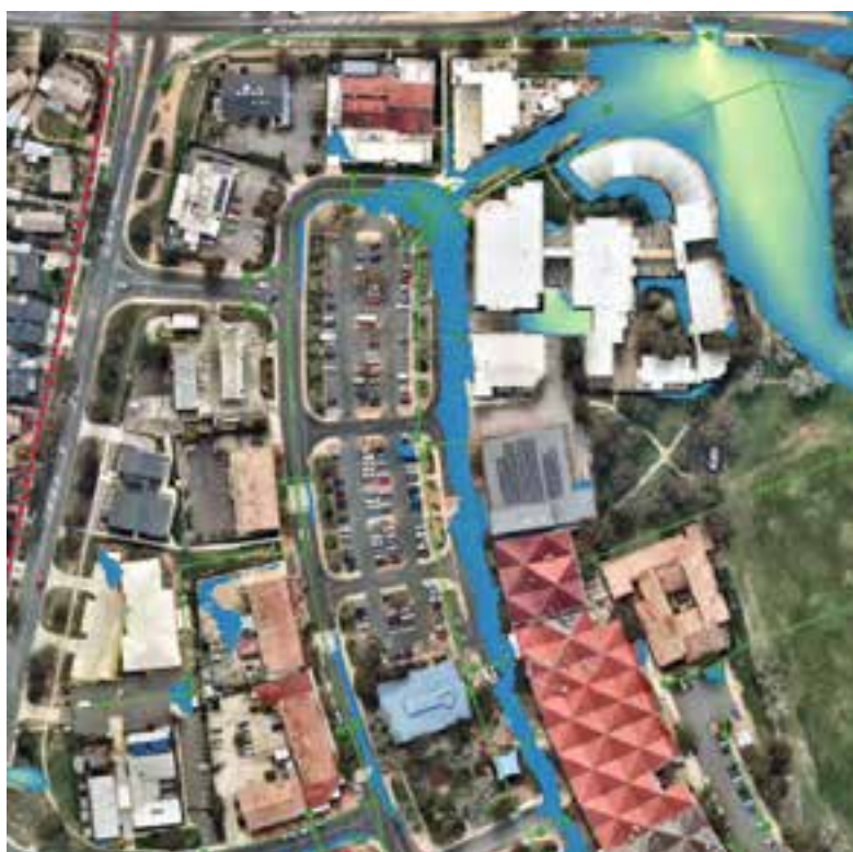
Figure 8-4 Peak flood extents along Hardwick Crescent during a 1% AEP 25 minute storm event
