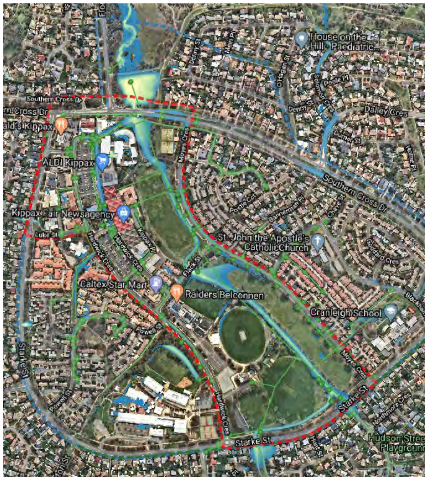
Figure 10-3 Mitigated 1% AEP flooding with 50% blockage
