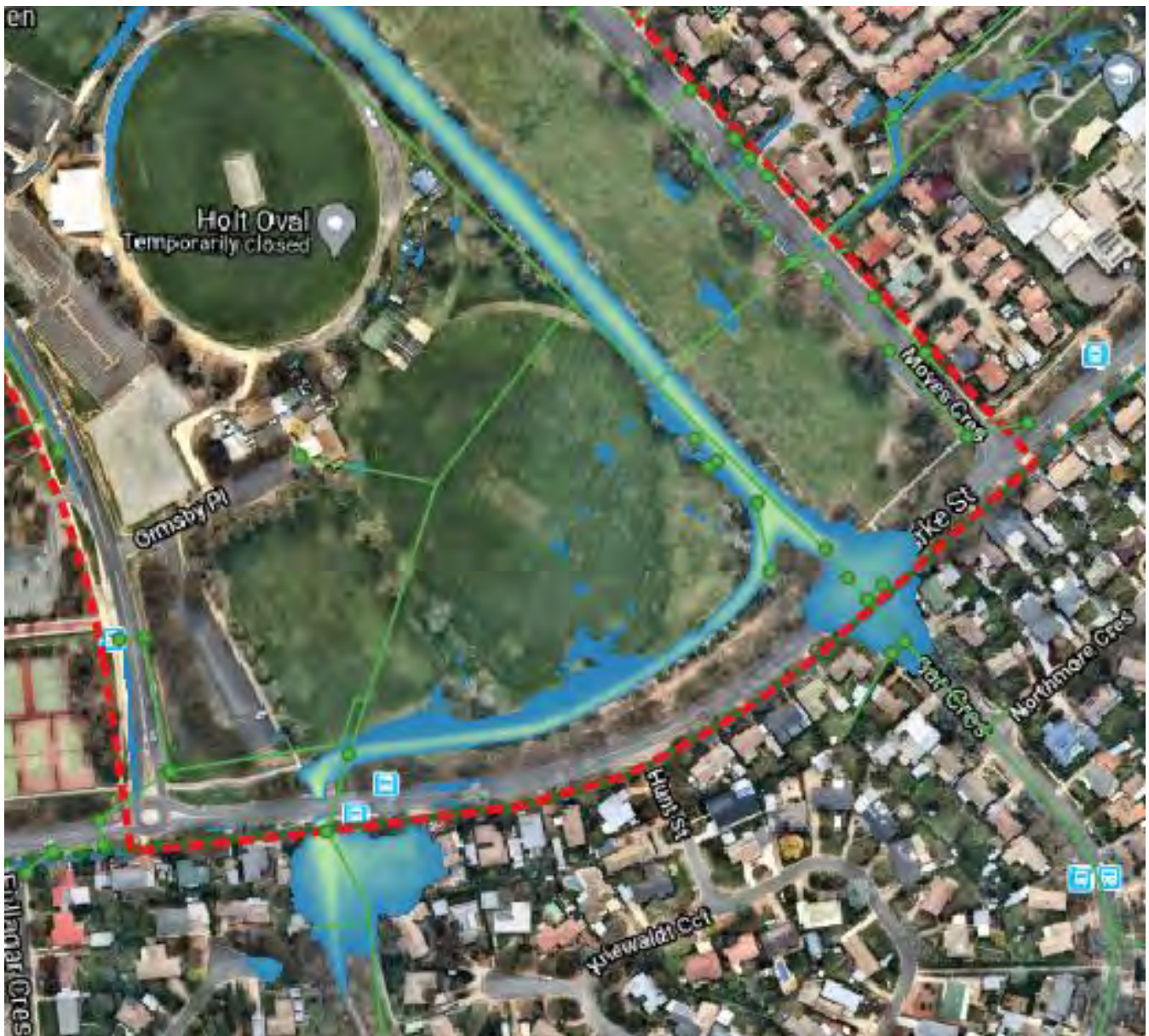
Figure 8-5: Peak flood levels of upstream and downstream of Starke Street Underpass during a 1% AEP 25 minute storm event
