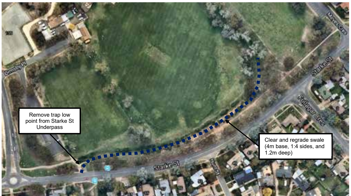
Figure 10-2 Mitigation Option – Clearing and regrading channel along Starke Street
