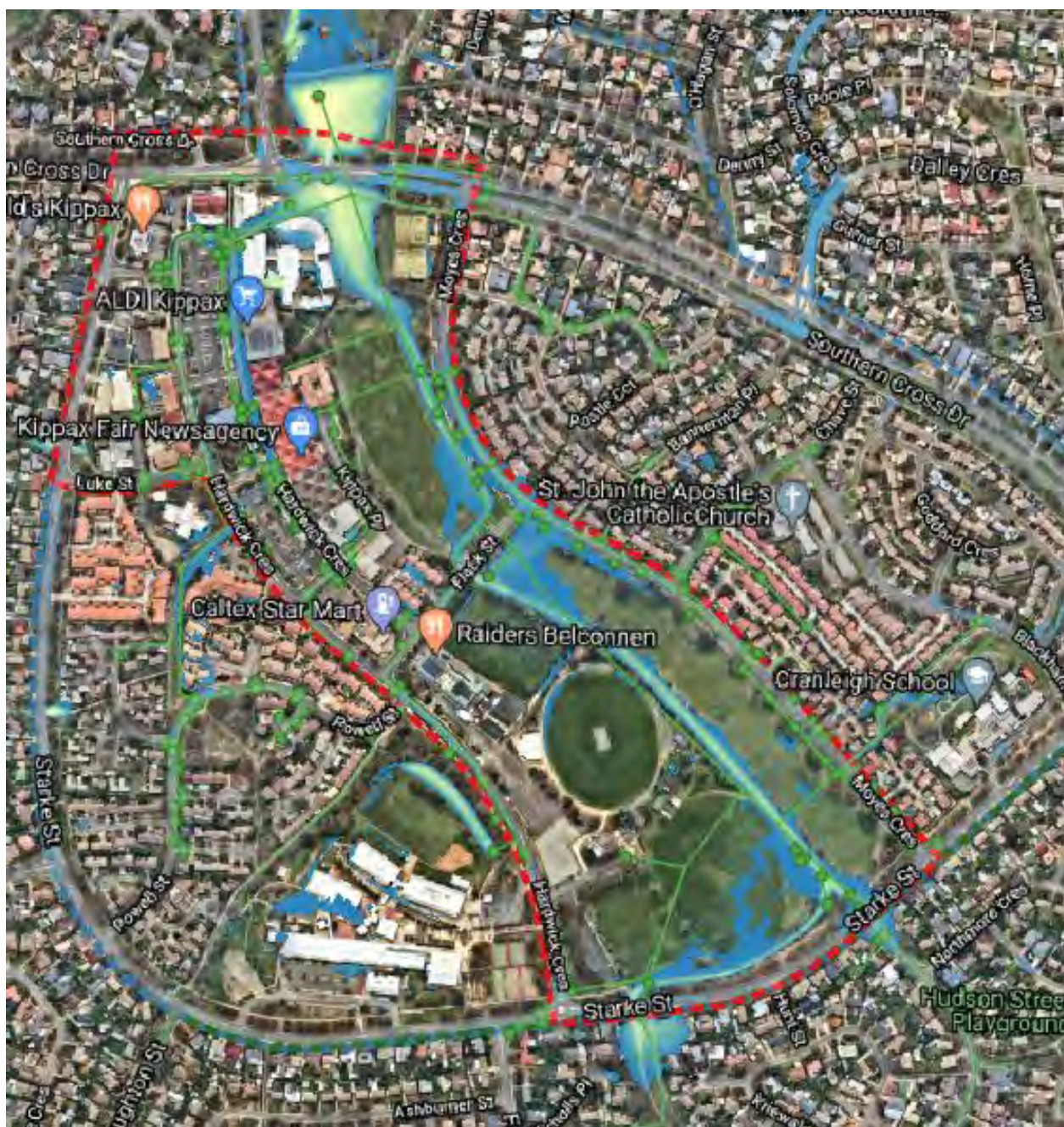
Figure 9-1: Peak flood levels with 20% increase to 1% AEP 25 minute storm event due to climate change
