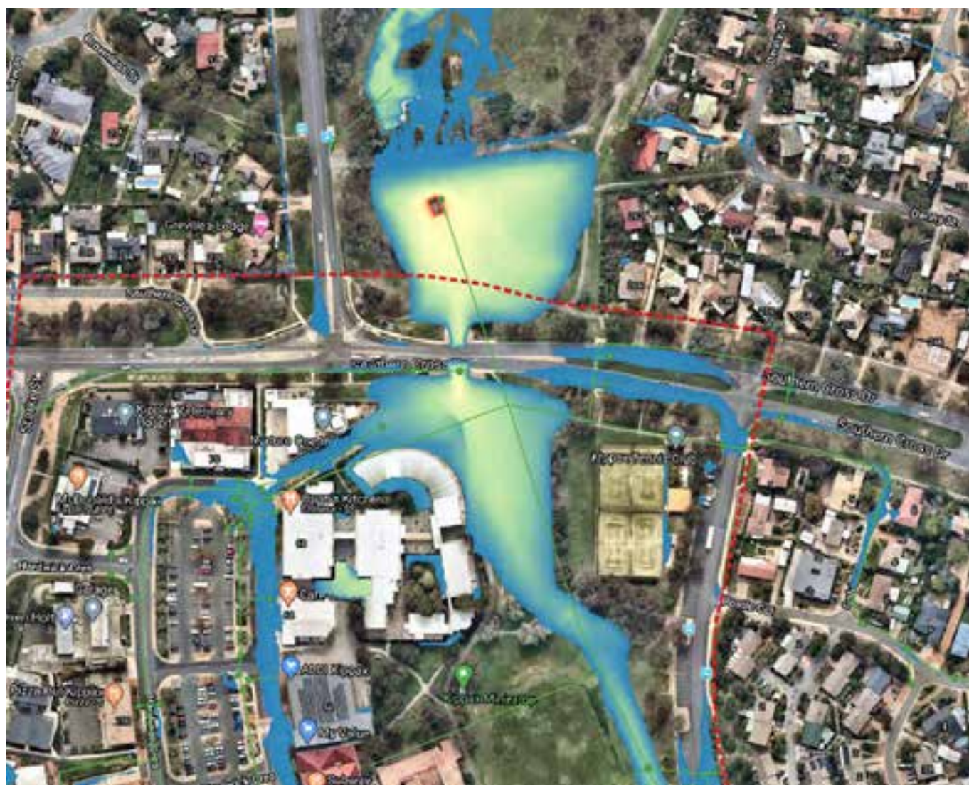
Figure 8-7: Peak flood levels at Southern Cross Drive during a 1% AEP 25 minute storm event
