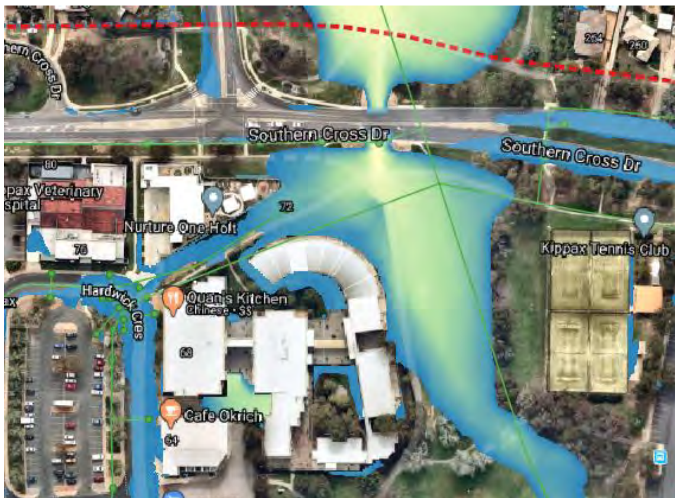
Figure 8-8: Flooding extent around buildings near Southern Cross Drive during a 1% AEP 25 minute storm event
