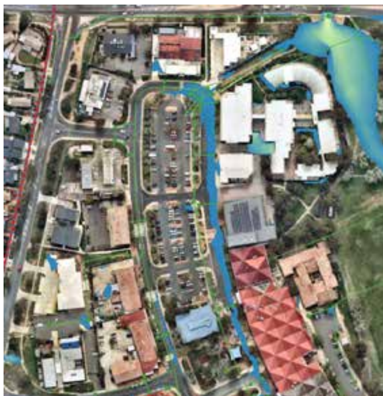
Figure 8-3 Peak flood extents along Hardwick Crescent during a 10% AEP 25 minute storm event
