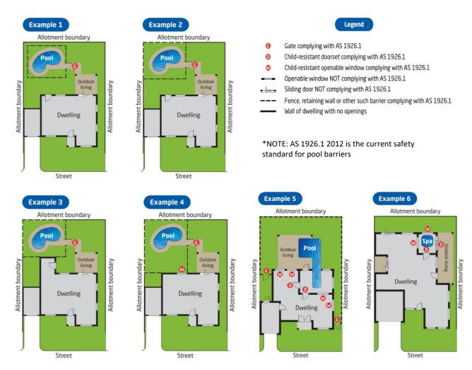
Diagrams for Barriers and Gates based on figures from AS 1926.1-2012.  $\ \odot$  Standards Australia Limited
