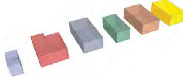
Modular Housing - Kit of Parts From L - R: Stair module; Garage (double or single) module; Living Area module, Main Bedroom module; Bedroom module; Bedroom + Study module
