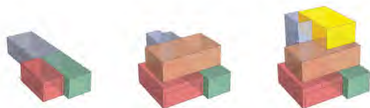
Modular Housing - Flexible arrangements Modules can be mixed and matched to form different combinations of accommodation. From L - R: 1 storey, 1 bedroom + single garage; 2 storey 3 bedroom + double garage; 3 storey 4 bedroom + study + double garage.
