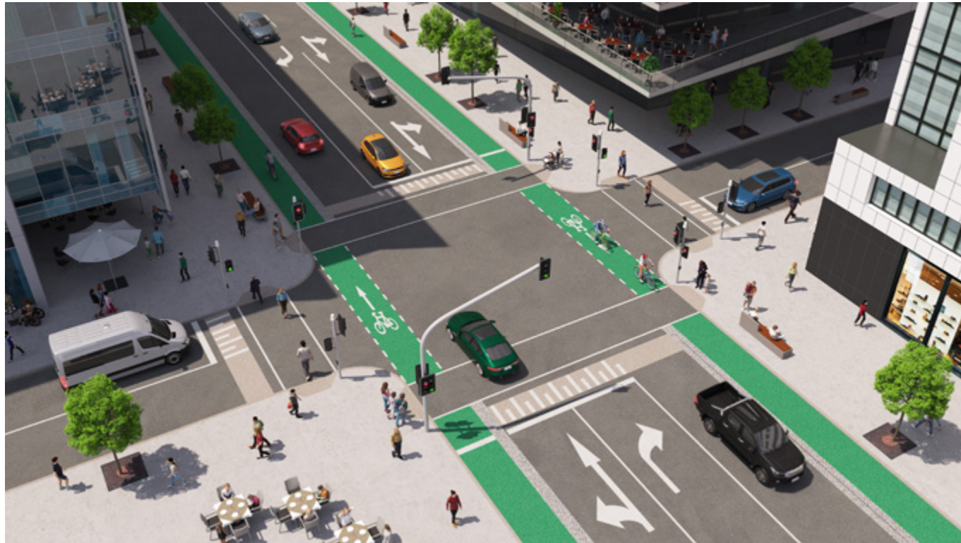
Figure 19 This collector to collector design is applied in a higher density setting. As such detailed road markings would be used. In a lower density residential setting, minimal road markings would be applied. In this setting protected lanes are only facilitated
