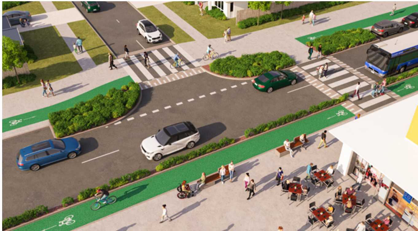
Figure 14 Bent out path where a local road meets a collector road [adapted from Cycleway Design Toolbox. Designing for cycling and micromobility (Transport for NSW, 2020)].
