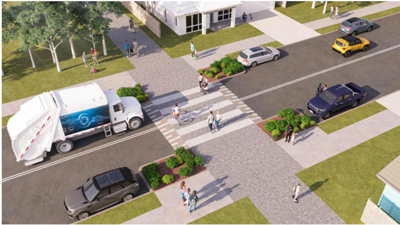
Figure 12 Local path network intersection with a local street, prioritising walking and cycling movements .
