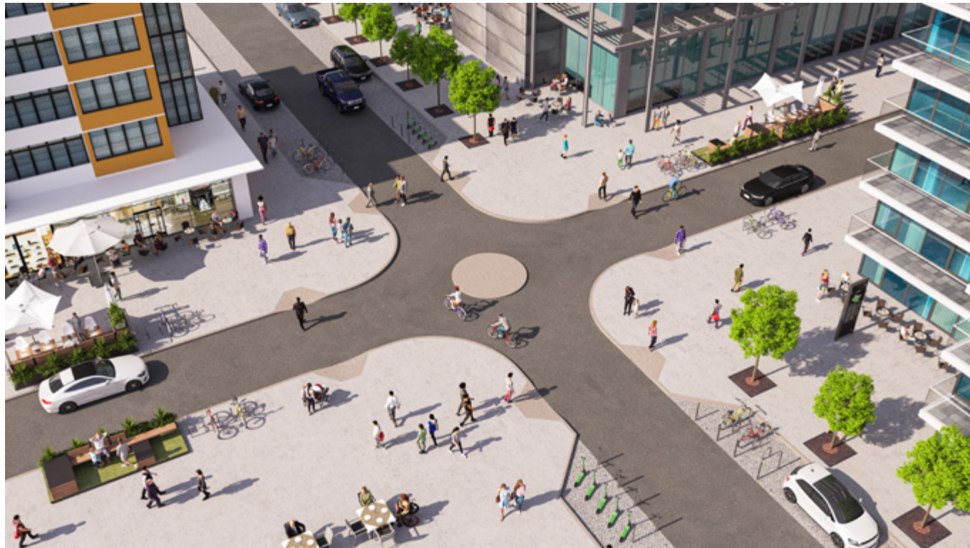
Figure 13 Local to local streets support local activities using short trips and therefore should prioritise active travel [adapted from the Urban Street and Road Design Guide (Auckland, 2022)].
