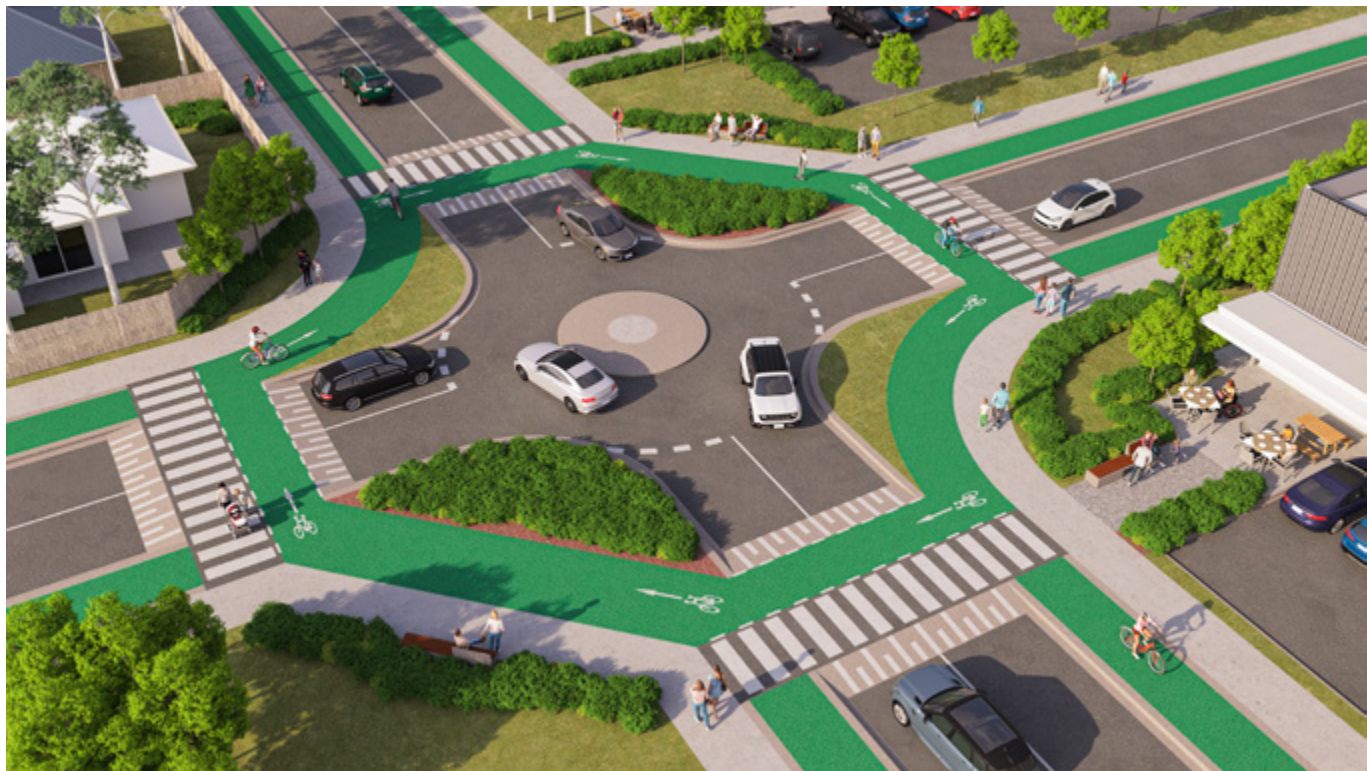
Figure 21 Tightened kerb radii slows turning traffic and increases visibility between road and path users (adapted from Cycleway Design Toolbox. Designing for cycling and micromobility [Transport for NSW, 2020]).
