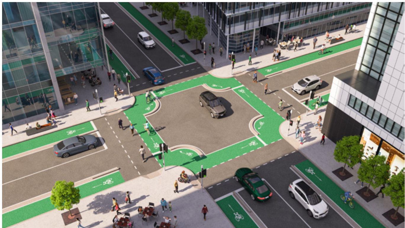
Figure 20 Collector to collector intersection where bicycle routes are present in both directions, [adapted from Cycleway Design Toolbox. Designing for cycling and micromobility (Transport for NSW, 2020)].
