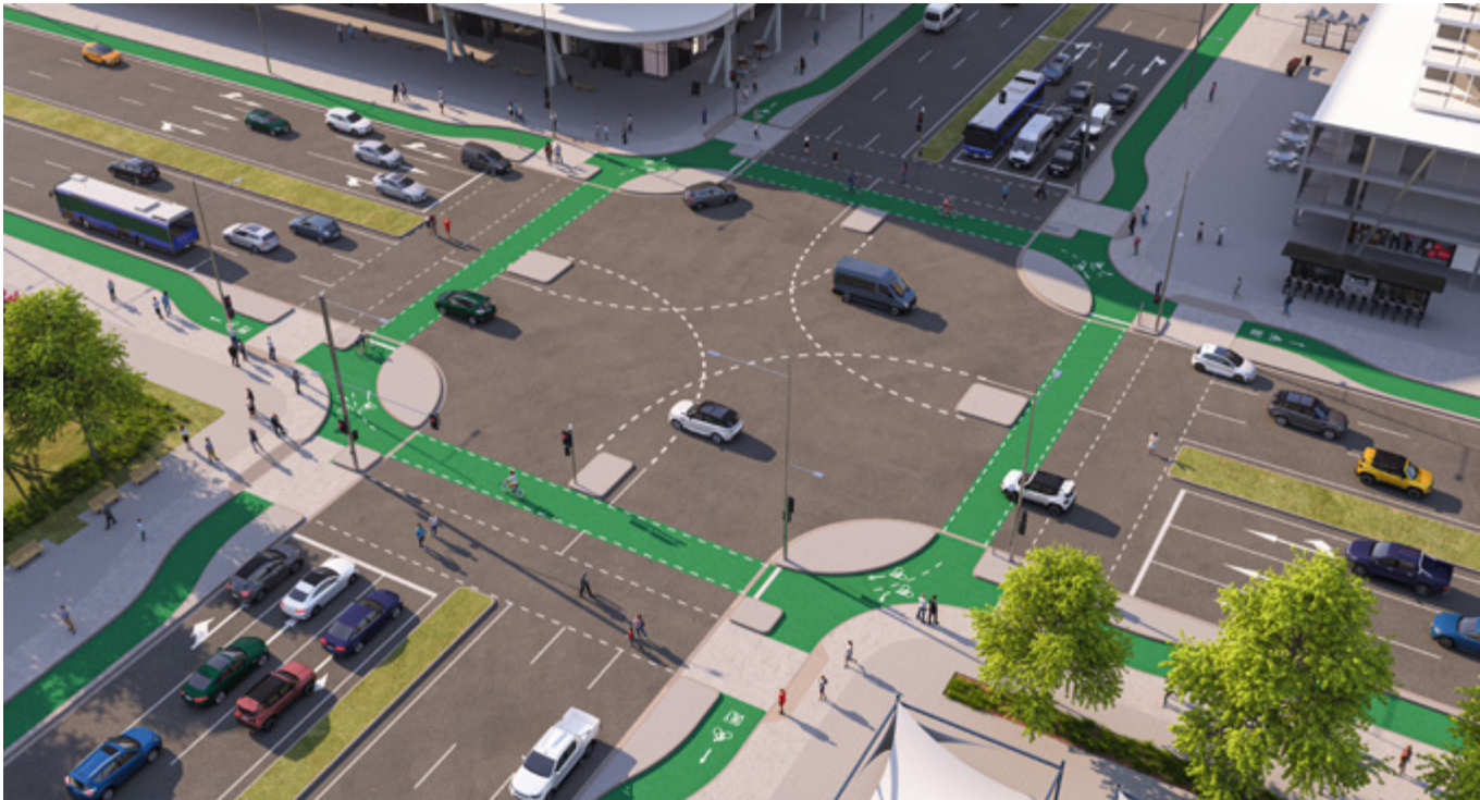
Figure 22 Arterial to arterial intersection with priority to active users [adapted from the Urban Street and Road Design Guide (Auckland, 2022)]
