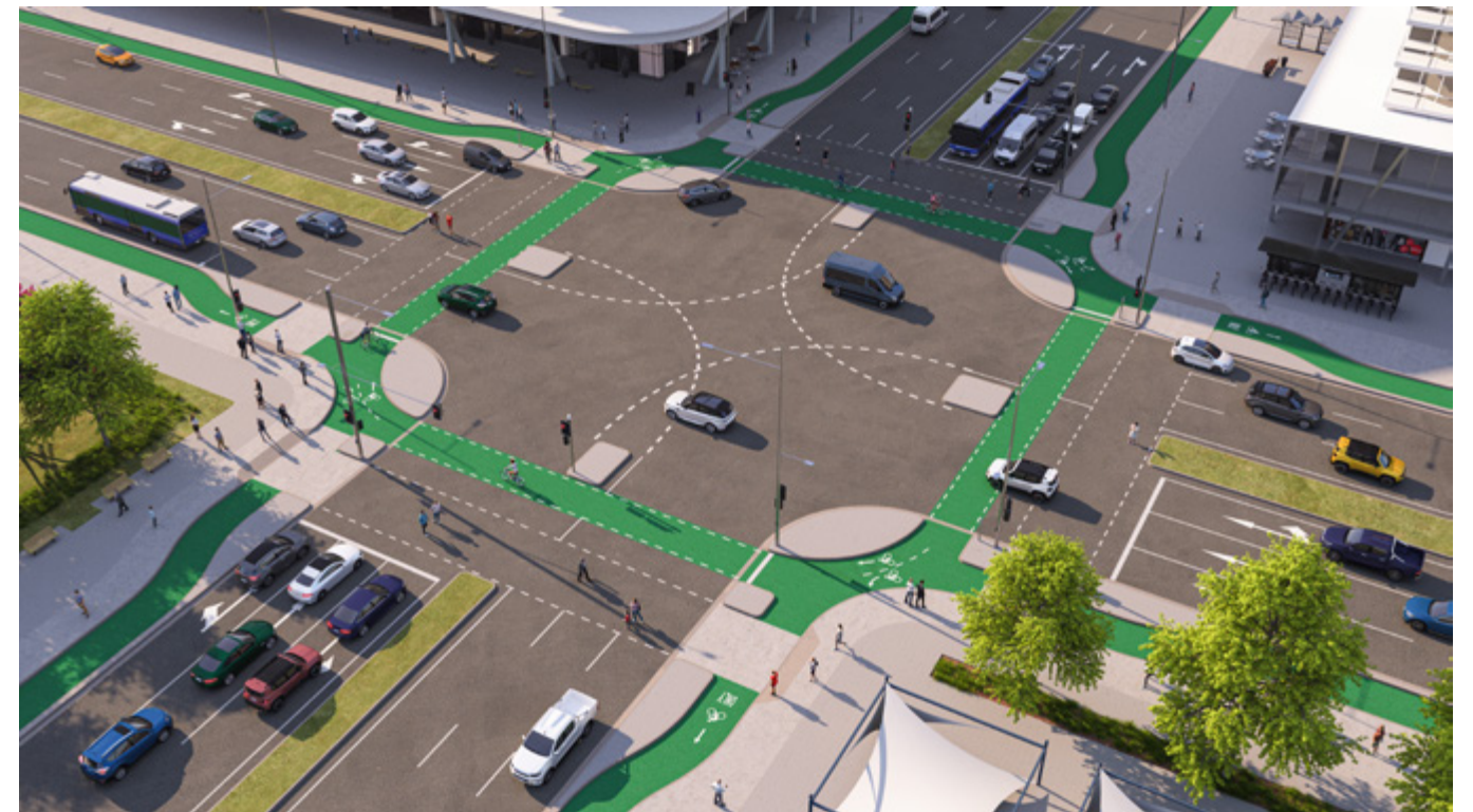
Figure 10 Signalised intersection. The principles set out in this diagram have been generally adopted in ACT Standard Drawing ACTSD-0561 and are discussed further in Section 5 [adapted from the Urban Street and Road Design Guide (Auckland, 2022)].
