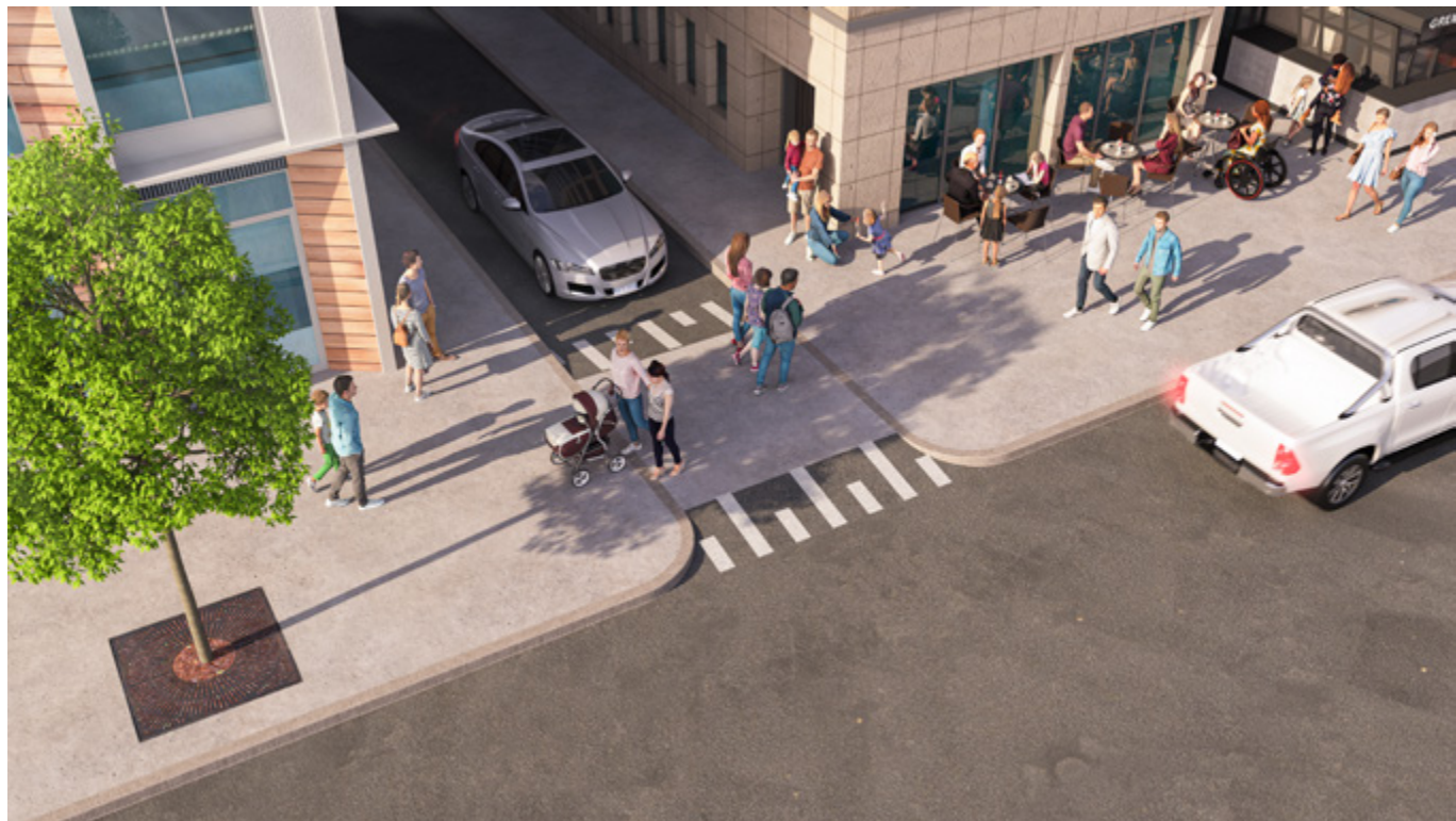
Figure 11 Priority crossing over driveways [adapted from the Urban Street and Road Design Guide (Auckland, 2022)].
