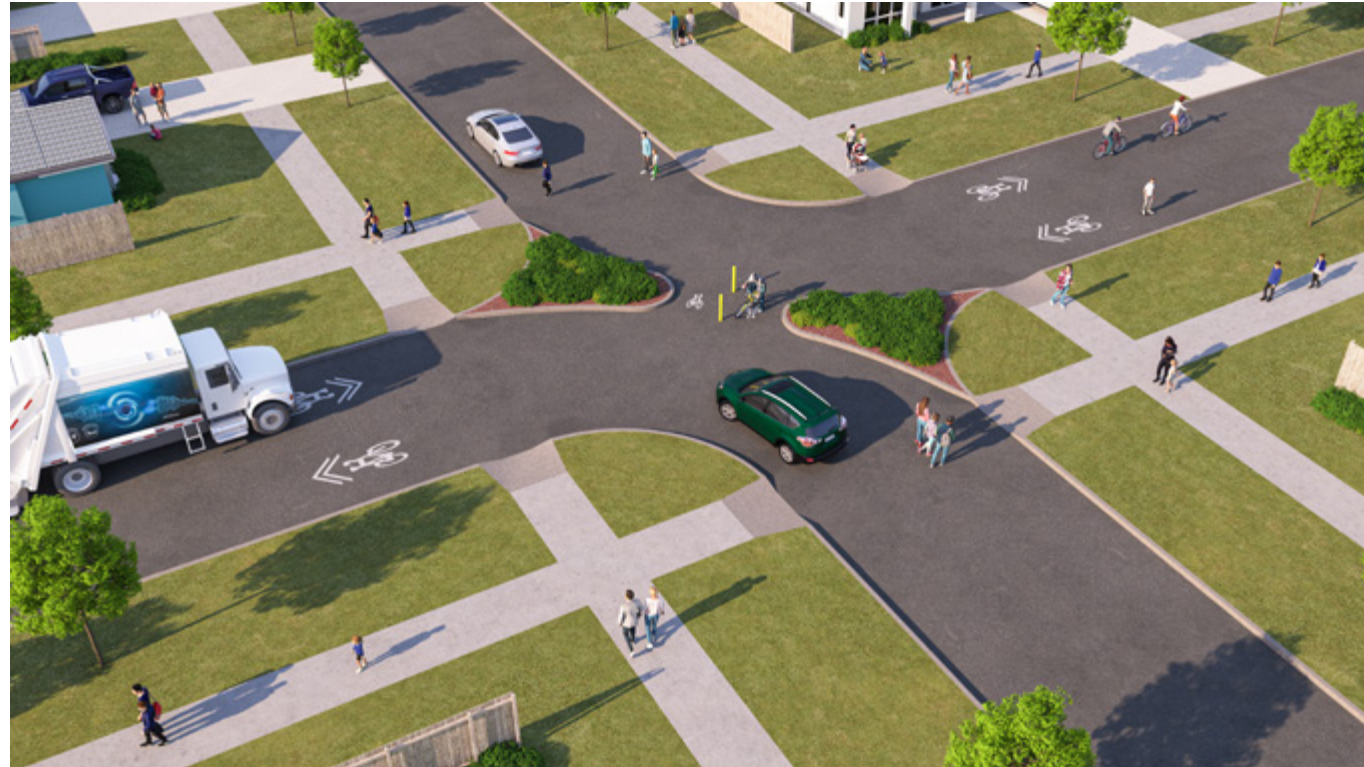
Figure 17 Treatment to reduce the number of intersections for cars and retain permeability for walking and cycling [adapted from the Urban Street and Road Design Guide (Auckland, 2022)]
