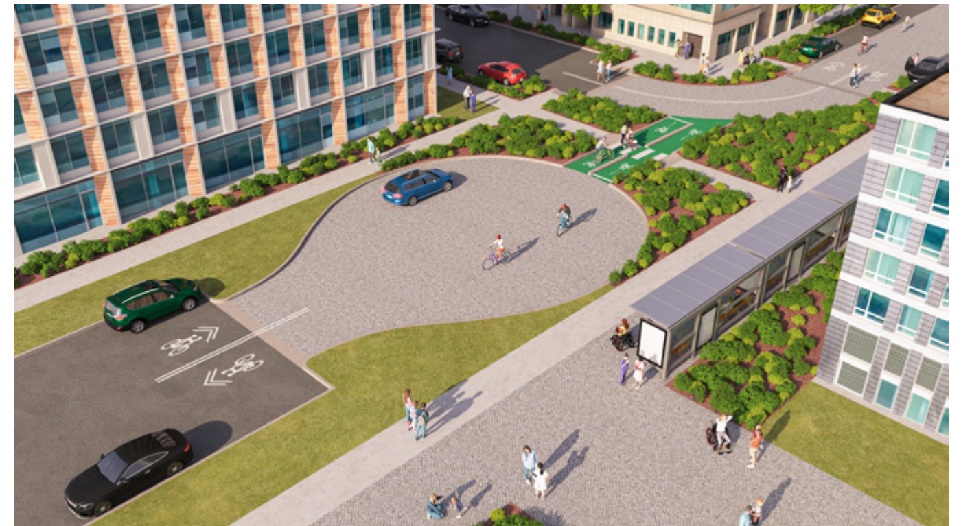
Figure 18 Modified T-intersection to restrict motor vehicle traffic and allow walking and cycling to filter through [adapted from Cycleway Design Toolbox. Designing for cycling and micromobility (Transport for NSW, 2020)].
