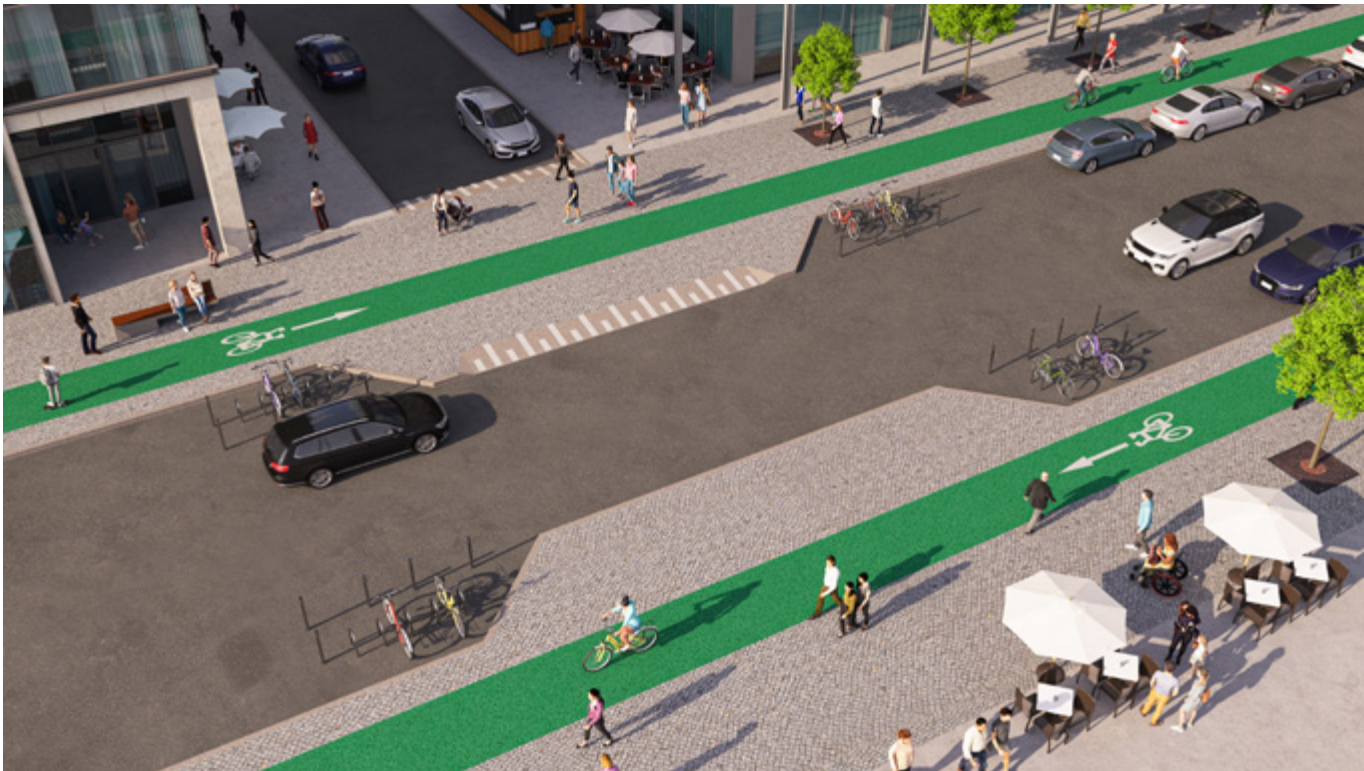
Figure 15 Priority path over laneways and local access streets in a busy inner-urban area [adapted from the Urban Street and Road Design Guide (Auckland, 2022)].
